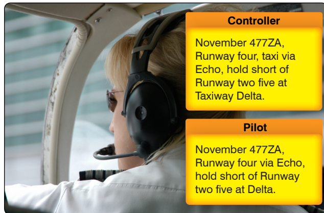
Figure 14-53. Example of taxi and “hold short” instructions from ATC to a pilot.
