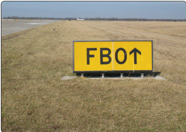
Figure 14-22. Destination sign to the fixed-base operator (FBO).
