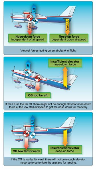
Figure 3-3. Center of gravity (CG).
