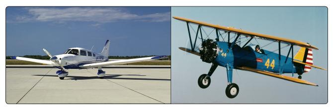
Figure 3-6. Monoplane (left) and biplane (right).
