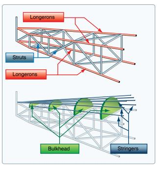
Figure 3-5. *Truss-type fuselage structure*.
