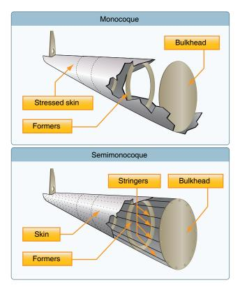
Figure 3-14. Semimonocoque and monocoque fuselage design.
