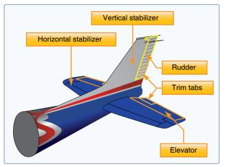
Figure 3-10. Empennage components.
