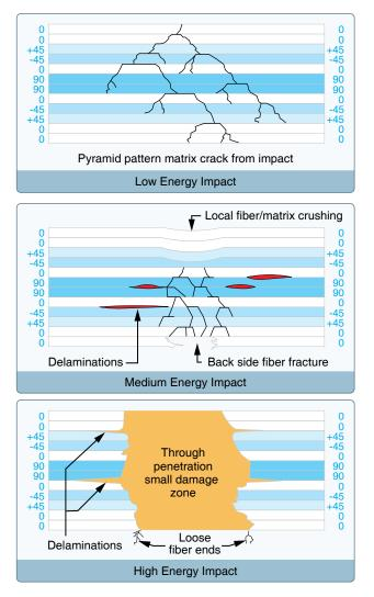
**Figure 3-16.** Impact energy affects the visibility, as well as the severity, of damage in composite structures. High and medium energy impacts, while severe, are easy to detect. Low energy impacts can easily cause hidden damage.
