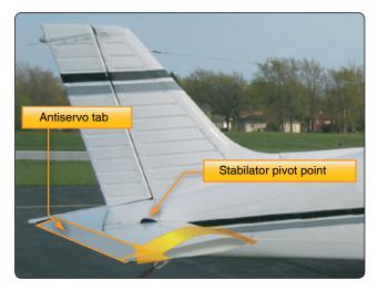
Figure 3-11. Stabilator components.
