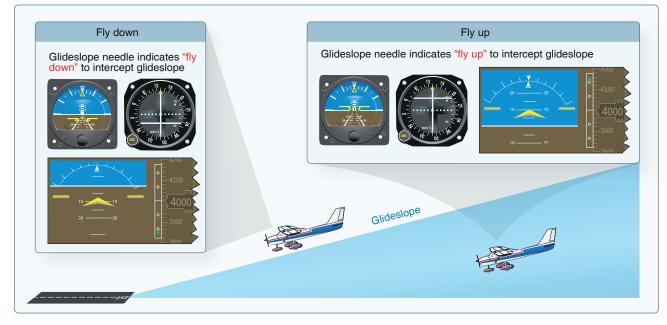
Figure 3-22. Analog and digital indications for glideslope interception.
