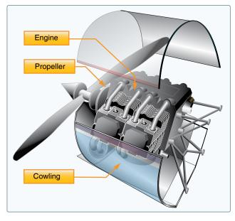
Figure 3-13. Engine compartment.
