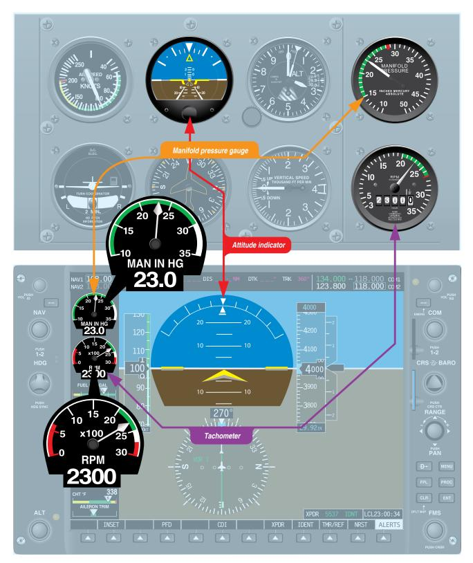
Figure 3-20. Control instruments.
